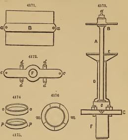
piston is filled with tow or some other soft material of a similar nature; the material thus inserted has a twofold use; in the first place, when saturated with sweet oil, it diminishes the friction that necessarily arises when the piston is forced through the ring mm; and in the second place, it prevents the admission of any extraneous substance which might increase the friction or injure the surface of the piston, and otherwise lessen the effects of the machine.
